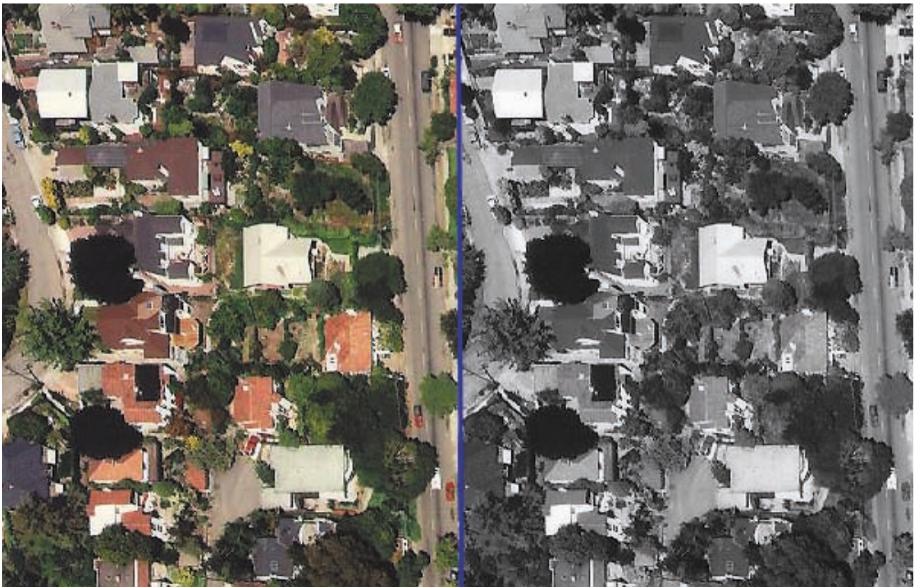
FIGURE 2.39 Comparison of black and white and color images of the same scene. Note how the increased number of tones found on the color image make the scene much easier to interpret. (Source: University of California at Berkley - Earth Sciences and Map Library)
