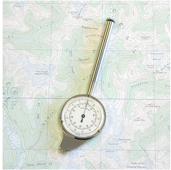
FIGURE 2.29 An opisometer is a mechanical instrument used to measure distance on maps. (Image Copyright: Michael Pidwirny)
