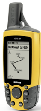
FIGURE 2.11 GPS receivers can determine latitude, longitude, and elevation anywhere on or above the Earth's surface from signals transmitted by a number of satellites. These units can also be used to reveal direction, distance traveled, and determine routes of travel in field situations. (Courtesy of Garmin)
