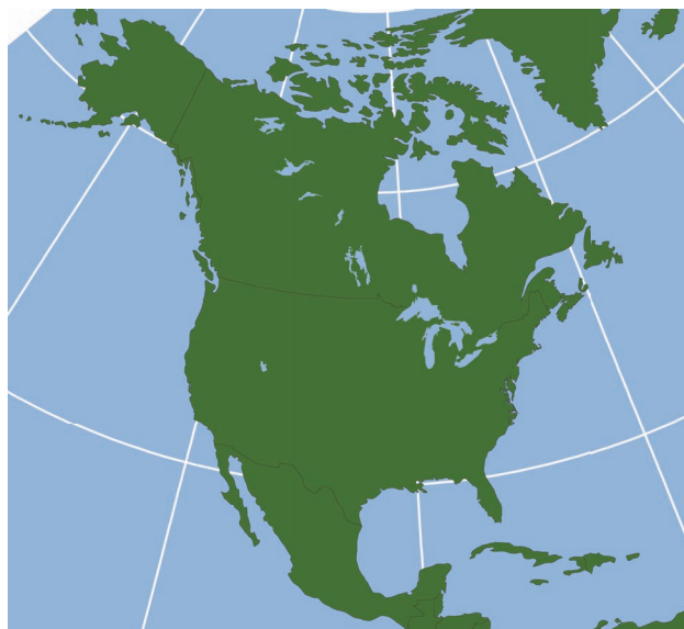
FIGURE 2.18 Map of North America created with the Albers Equal AREA PROJECTION. his map uses two standard parallel in the projection process: 20 and 60° North. Distances are true only along these lines of latitude. Areas are proportional to the same areas on the Earth's surface. Directions are reasonably accurate in the regions around the standard parallels. (Image Copyright: Michael Pidwirny)
