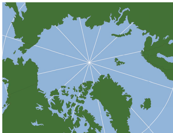
FIGURE 2.20 Map of the region around the North Pole. This map was created with a Gnomonic planar projection. In this projection, lines of longitude appear as straight-lines that radiate out from the North Pole. Lines of latitude appear as circles. Scale distortion increases rapidly away from the central point (North Pole) of this projection. This map can be used by navigators to find the shortest path between two points. (Image Copyright: Michael Pidwirny)
