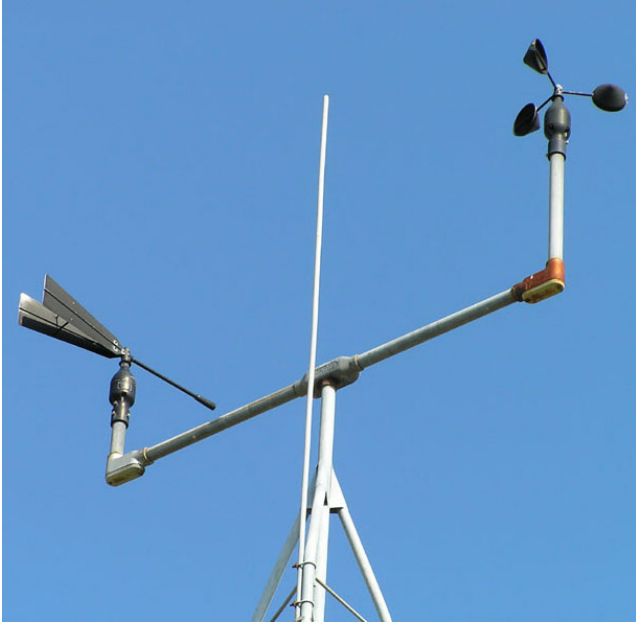
FIGURE 7.12 Wind speed is commonly measured with an anemometer. An anemometer consists of three open cups attached to a rotating spindle. The speed of rotation is then converted into a measurement of wind speed. Wind direction is measured with a wind vane. On the photograph above, the wind vane instrument has a bullet shaped nose attached to a finned tail by a metal bar. (Source: NOAA)
