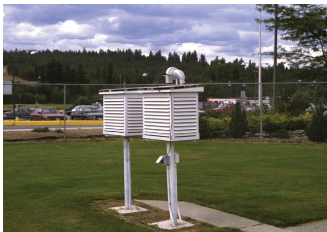
FIGURE 6.5 Stevenson Screen meteorological instrument shelters. These shelters are typically made of wood, painted white, and have louvered sides. They also are elevated to height of about 1.5 meters (about 4.5 feet) by a wooden or metal base. Some instrument shelters have an electric fan attached to them for better air circulation in the instrument box during light wind conditions. (Image Copyright: Michael Pidwirny)
