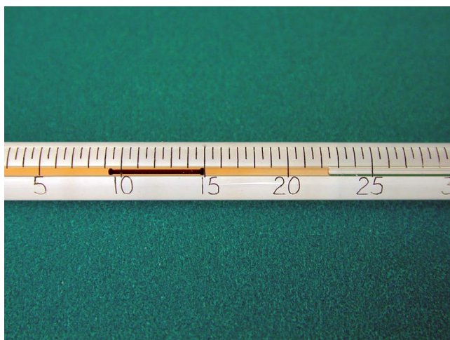
FIGURE 6.4 The minimum thermometer measures the lowest temperature over a specific time period with a metal slider located inside the bore of the thermometer. The surface tension that exists at the top of the alcohol column moves the slider as the temperature drops. When temperature increases the slider does not move with the expanding alcohol. In this example, the recorded minimum temperature is 15^{\circ}\text{C} . Note that the current temperature is about 22.5^{\circ}\text{C} . (Image Copyright: Michael Pidwirny)
