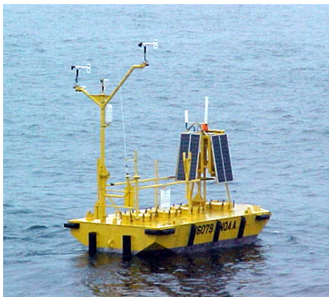
FIGURE 6.26 Remote weather station buoy with a 6-meter boat shaped hull. (Source: NOAA)
