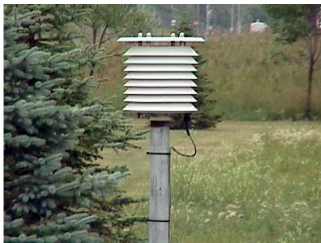
FIGURE 6.5 The following meteorological instrument is called an Electronic Maximum and Minimum Temperature System (MMTS). These systems consist of three main parts: a white ventilated instrument shelter, an internal electrical thermistor, and a computerized data storage device (data logger). Thermistors are a type of thermometer that measures temperature based on the fact that electrical resistance of a conductor varies with temperature. Thermistors can provide a continuous digital record of temperature change. From this record, maximum, minimum, and mean temperatures can be determined daily. The U.S. National Weather Service is replacing the older liquid-in-glass thermometers with the Electronic Maximum and Minimum Temperature Systems at many of their primary and cooperative observing stations. (Image Copyright: Michael Pidwirny)
